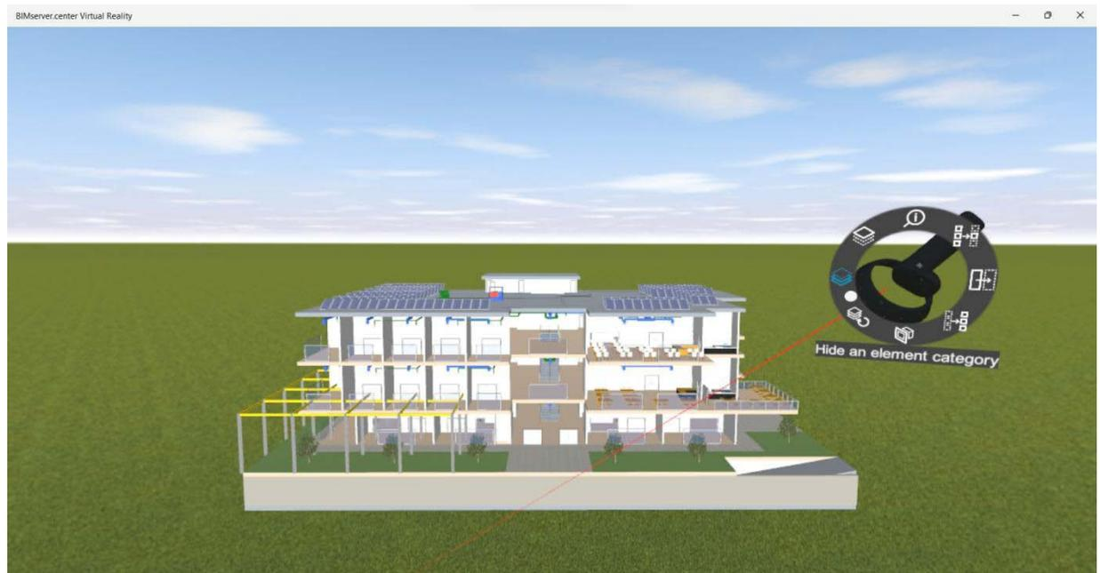
The image shows the selection of the external envelopes of the model (façade, louvres, etc.), hiding these element categories.
