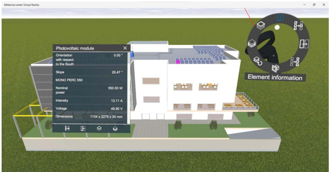
The image shows the BIM information of a PV module from the project, using the tool described above.
